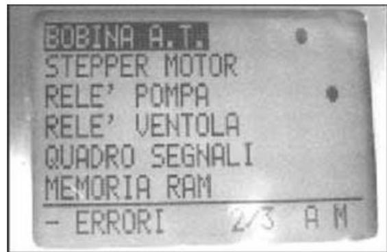
**11** - There is also a fault message for the HV coil.
