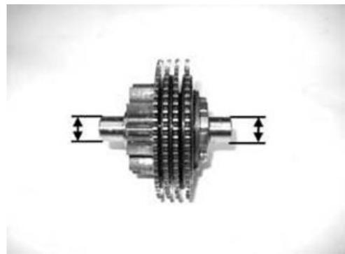
Also check the shaft diameter on the flywheel cover and on the engine crankcase.
