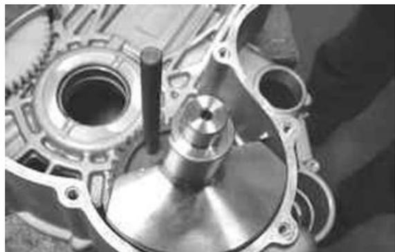
**Specific tooling****020471Y Pin for countershaft timing**
