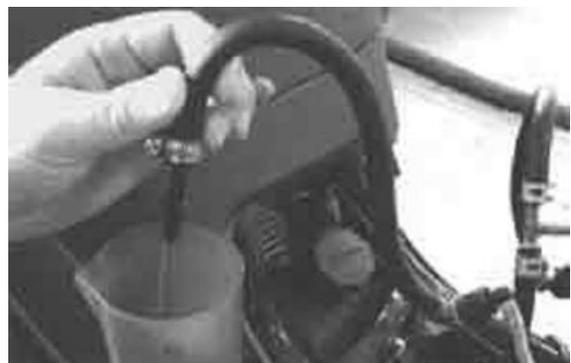
**17** - Introduce the return pipe into a graduated container.
