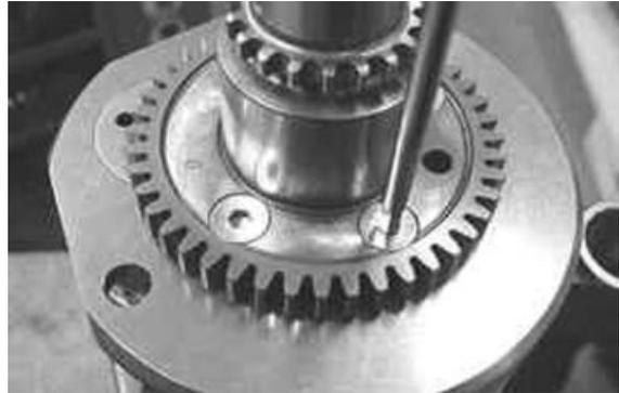
Blow with compressed air and degrease the mounting holes on both surfaces to make the new LOCTITE grip.
