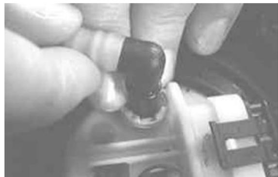
The system pressure check must be carried out, for practical reasons, by connecting on the pump side.
