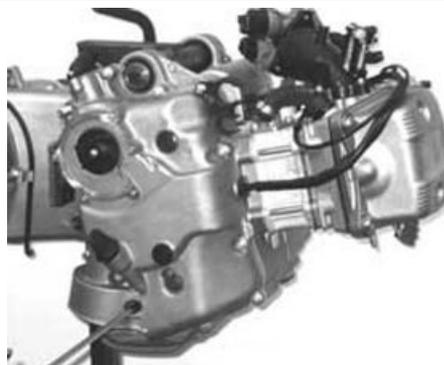
**Removing the intake manifold**
