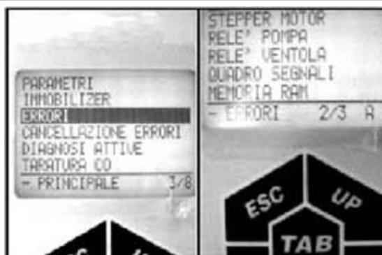
2 - Select the menu on the "ACTIVE DIAGNOSIS" function. Activate the electric fan diagnostic function. Check acoustically for rotation of the electric fan. Wait for the exit from the diagnostic tester.
