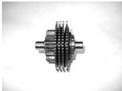
The limiter assembly cannot be overhauled. In case of irregularities on the toothed discs, replace the assembly.
